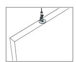
Suspension with Connect Adjustable wire hanger
