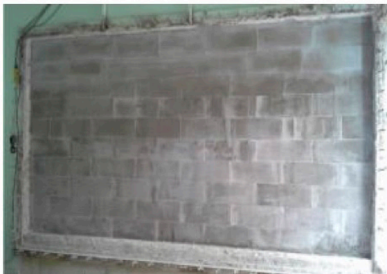
Tested wall with gypsum mortar
